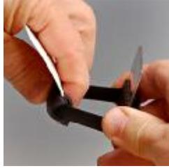
Pull the reflector and mirror apart so the elastic is stretched as shown.
