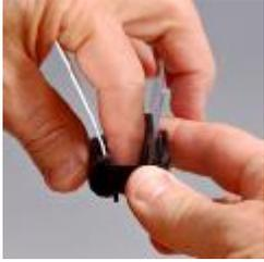
Hold both sides of the mirror with your right hand and insert your left forefinger between the reflector and the mirror.
